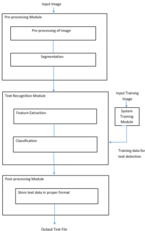
Fig. 1. Block Diagram Of Text Recognition
